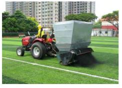
Install the platform and brushes on the machine and perform a test run to check everything is functioning. Always perform this test run next to the field to prevent any possible damage to the field through oil leakage.
